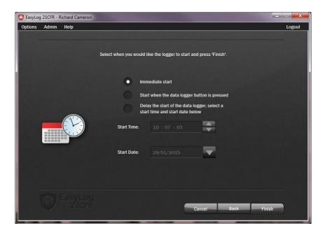
The data logger can be setup to start in three different ways:
