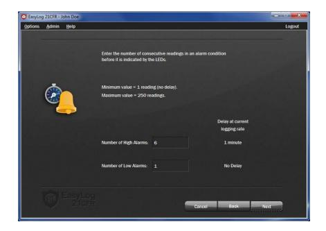
Some of the data loggers have a function to delay an alarm from triggering. In some situations you may not want to show an alarm on the LEDs until several consecutive alarm readings have been gathered. Perhaps a single alarm condition log doesn't warrant any corrective action but several logs in alarm mode might. In these instances, it is possible to delay the LED indication by a user-selectable number of logs in alarm mode.
