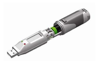
Slide the two parts of the data logger enclosure back together again, until a click is heard. This confirms that the two parts are snapped together correctly.
