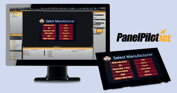
The SGD 70-A is a PanelPilotACE compatible display designed specifically to run projects created in the PanelPilotACE Design Studio. It features a capacitive touch screen and a wealth of hardware interfaces including four 16-bit bipolar analogue inputs, eight digital input/output pins, two alarm outputs, four PWM outputs, RS232 and RS485 comms, CANbus and FTP transfer of logged data via Ethernet.
