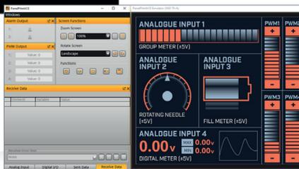
Design Studio's Preview Emulator, which emulates the hardware inputs and outputs, allows students to test their display projects before uploading anything to an actual display.
