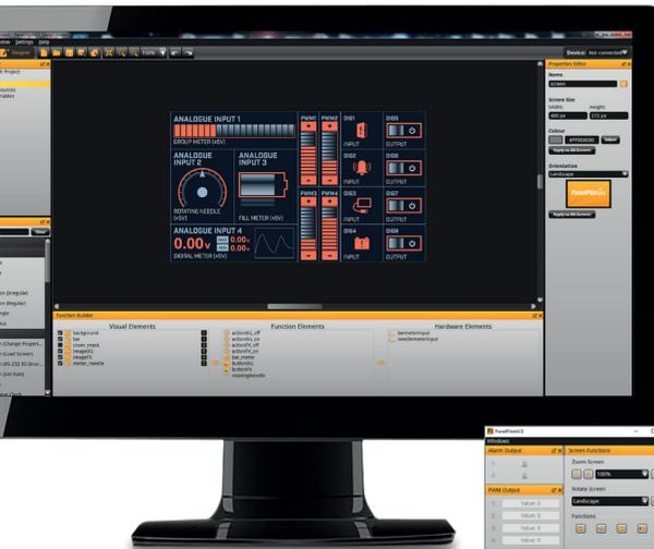
Hardware elements are dragged from the library into a function builder where associations with graphical elements (such as a needle on a meter) can be defined.
